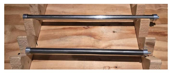
To decouple the two rods joined by attraction force, first rotate one slider by 90 degrees to reduce the force, and then complete the decoupling by applying the necessary separation force.
