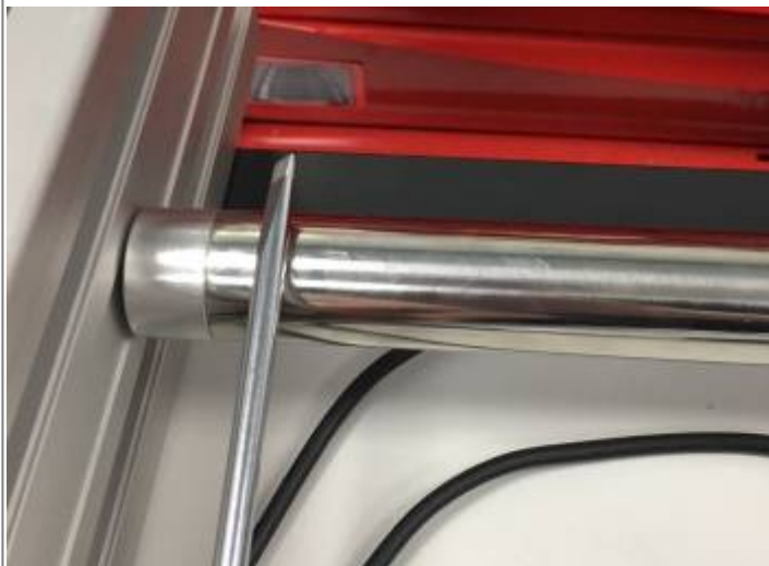
Position when the magnets start. (close to the shaft end) Yellow point is on this side
