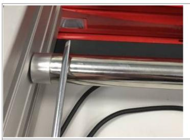
Position when the magnets start. (close to the shaft end)
