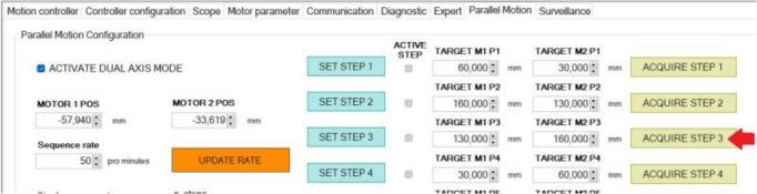
Move the robot in the starting position and store the forth positions using ACQUIRE STEP 4 button.
