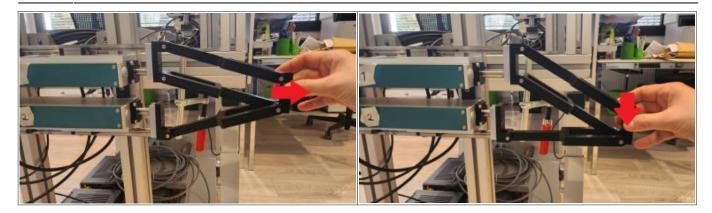
Press button Acquire Step to capture the position of the two axis. If the number are with digits you can correct using the number field and press the SET STEP 1 to store.
