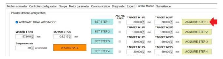
Move the robot in the push position and store the second positions using ACQUIRE STEP 2 button.
