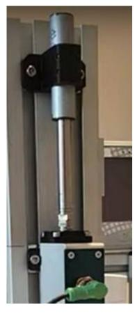
In vertical applications, when the rotolinear motor is not powered, the linear axis can fall down due to gravity. Using MagLift, the gravitational force is counterbalanced and the linear motor remains in steady state. 6 force sizes are available: 12, 17, 22, 40, 50 and 60 N, respectively MagLift12, MagLift22, MagLift40, MagLift50 and MagLift60.
