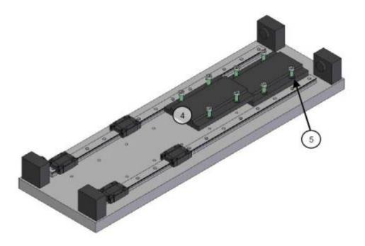
3: Mount and secure the motor assembly (6) on the linear guides (7). Warning: pay attention to leave a minimum gap of 5 cm between the magnetic way and the motor assembly in order to avoid unintentional movement of the motor assembly.
