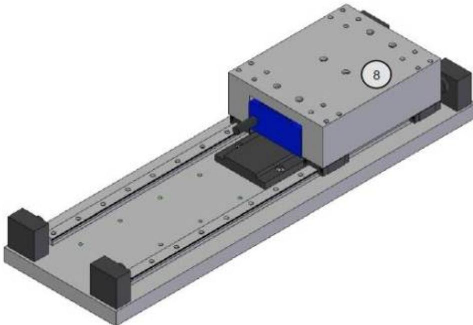
5: Mount and secure the remaining magnetic way segments (9) with the fixing screws (10). The segments must be oriented with the north pole in the same direction; the position of the north pole is indicated on the name plate with N.
