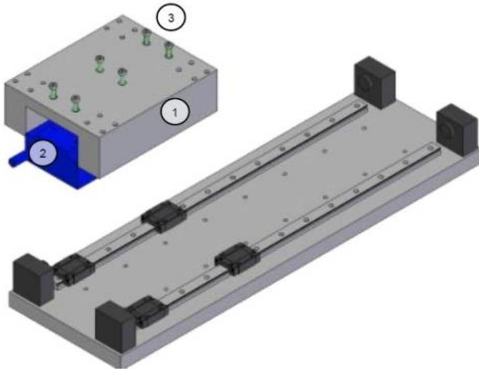
2: Mount and secure the magnetic way segments (4) on the baseplate with the fixing screws (5). The segments must be oriented with the north pole in the same direction; the position of the north pole is indicated on the name plate with N.
