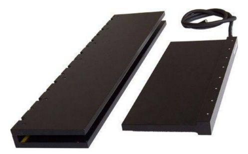
Synchronous linear motors with a primary part without ferromagnetic materials The primary parts of these linear motors are characterized by low weight, practically zero attraction forces between the primary and secondary parts, high efficiency and the absence of traction force pulsations (cogging). Thanks to these properties, they can be advantageously used in dynamic applications demanding feed rate, acceleration, precision and low weight of the drive.
