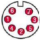
Male, 7-pin (D70) integral connector (pin-out as viewed from the end of the sensor)
