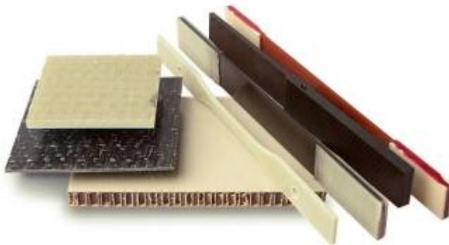
Composites are complex materials made from polymers reinforced with a fiber such as glass, aramid, or carbon. They are used extensively in applications such as aerospace and wind energy that demand high strength, lightweight materials. Key composites testing standards include ASTM D3039 and ISO 527-4. Important measurements include tensile strength, shear strength, yield strength, and fracture toughness.
