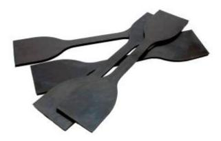
Elastomers are high-elongation materials such as natural rubber, silicone, and polyurethanes that are used for making tires, medical devices, sealants, and many other products. Tensile strength, total elongation, and tensile stress at a given location are key properties. Major testing standards include ASTM D412, ASTM D642, and ISO 34.
