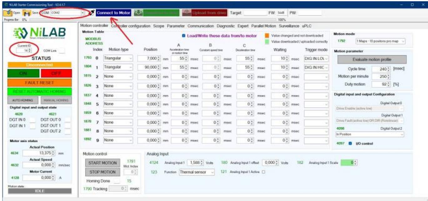
Check if the motor is running with the previous configuration of the replaced motor.
