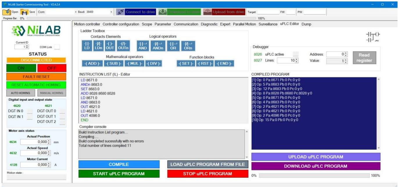
The IL compiler check for syntax and logical error and then compiled the program for the internal PLC. After the building phase the user must download the program into the motor using the DOWNLOAD button.
