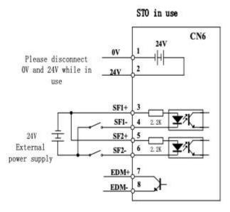
Please take precautions when enabling STO functions as servo drive will lose control over the motion of the motor. Motor might dropped under gravitational pull (vertically mounted load) or moved when external forces a re applied to it. Alternatively, motor with holding brake can be chosen.
