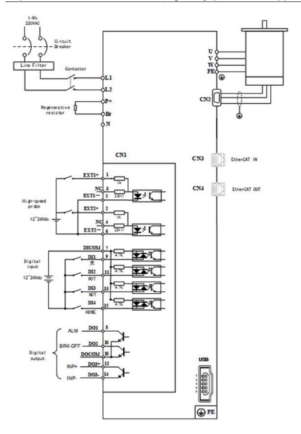
NL7-RS series servo drive supports single phase and three phase 220VAC. Only driver with power rating above 1500W supports three phase 220VAC.
