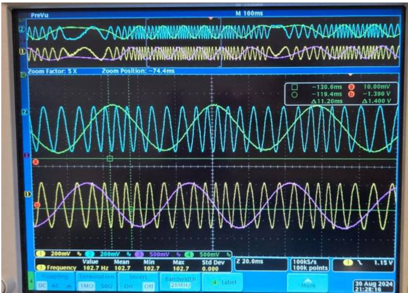
Example of SIN/COS Output (Blue and Yellow) with the encoder configured with 2mm of sine period.
