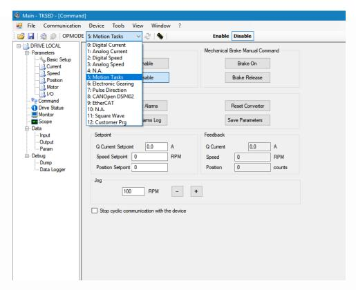
Then select the Diagnostic mode to use the Motion task debug window. Go to Administration and set the password **fpcb**.
