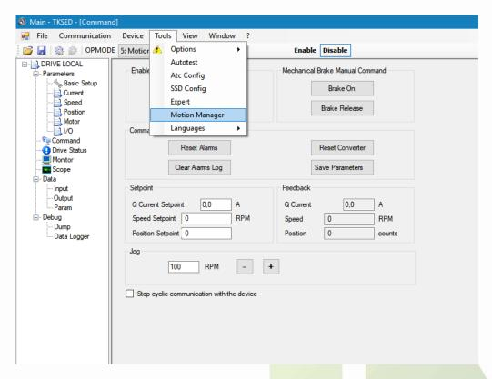
Using the motion manager you are able to set the bit of the control word manually to start homing and the sequence.
