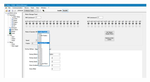
Then the most simple way is to do homing is select the homing method to 35. Current position
