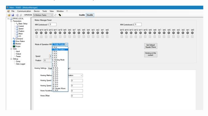
Then enable the drive clikking on bit0 and then on bit4 to start the sequence.
